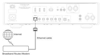
Connect a network cable (Category 5/5E straight through Ethernet cable) between the 851N and your router.
