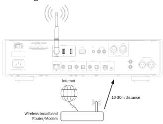
Connect the supplied wireless dongle to the correct USB input on the rear of 851N – it will need to be in range of your wireless router.
